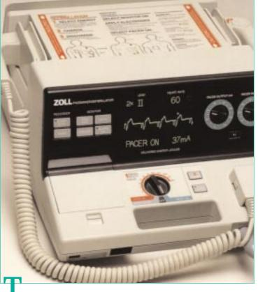
he ZOLL PD 1200, combining defibrillation, pacing, and monitoring, offers complete ACLS-response capabilities in a single, easy-to-use unit that is ideal for critical and speciality-care areas. It can be configured with the ZOLL "hands-off" Multi-Function Electrodes, with standard defibrillation paddles and pacing electrodes.
